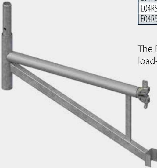
The RINGSCAFF side brackets are designed for a maximum load-bearing capacity of 1.5 kN/m<sup>2</sup> on the extended platform.
