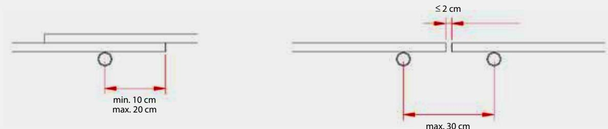
Figure 5.6: Arrangement of the wooden planks
