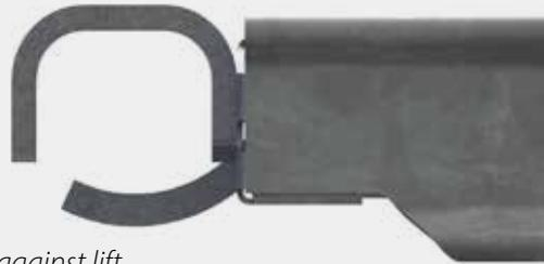
Figure 5.2: Securing the steel decks against lift
