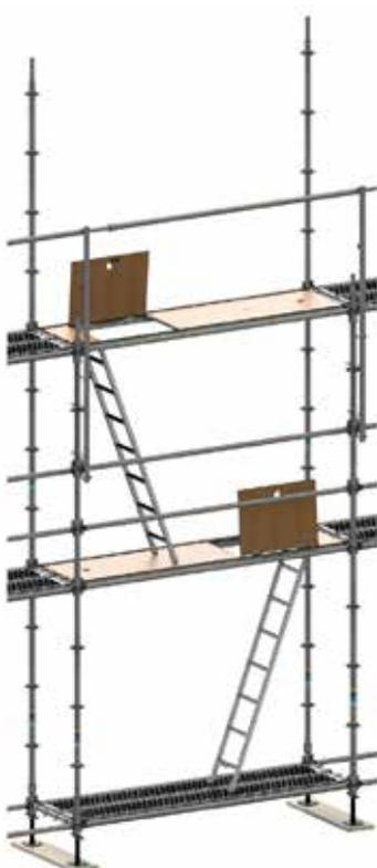
Figure 8.19: Fitted mounting safety guardrail (MSG)
